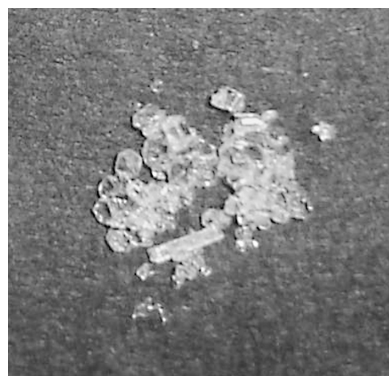
Figure 2. Photographic image of the recrystallized Al(acac) 3 . 1 H NMR of CDCl 3 solution exhibits two singlets at δ = 1.99 (6 H, s, C(O)CH 3 ), and 5.48 (1H, s, C(O)CHC(O)) that are consistent with the chelating acetylacetonato ligands.
